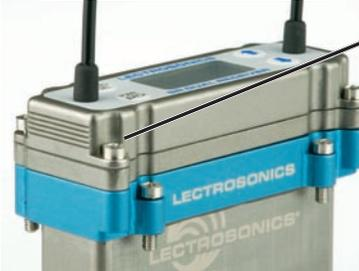
Slide the adapter up and tighten the retaining screws to secure it to the receiver flange.
