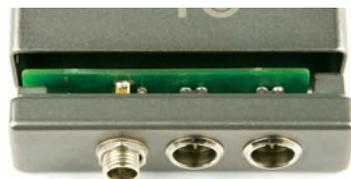
Carefully align the mating connectors and gently slide the panel straight into the housing until the screw holes align with the housing.
