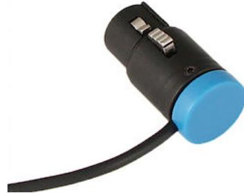
4. You can loosen the Grub screws and carefully twist the cap between the screws to align the cable exit to your preference. If you need the exit to be on the opposite side of the connector, e.g. Exit off of PIN 2 instead of PIN 1, you will need to remove the cap and bend the cable assembly carefully towards the other side. If you just remove the screws and twist the cap all the way around to the other side you will have a bad day.
