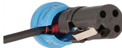
3. Place the insert into the XLR shell and bend the cable towards the position you would like the cable to exit the cap. Install the color cap. Carefully pull the cable so the Zip-tie rests against the inside of the cap exit. Install the Grub screws with the included Hex wrench while applying constant pressure to hold the cap in place. DO NOT OVERTIGHTEN! You only need to torque the screws to the point where the screw is flush with the outer shell. Overtightening can damage the color cap.
