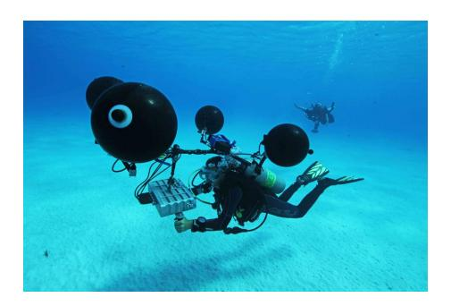
SD-UW: Underwater housing for Sound Devices 7-series recorder
