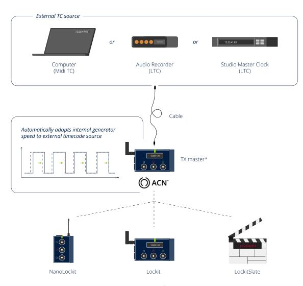
\* Can be any Lockit device started up with  $\bigcirc$  **Red** +  $\bigcirc$  **Power**. We broadcast Start, Stop and Freeze Frame through ACN.
