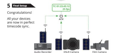
Timecode from an external source can now be sent from one device to other devices. This external source must be permanently connected to this Nanol ockit via TC input or MIDI USB.
