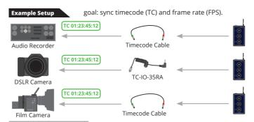
NOTE: Required cable depends on connected device.
