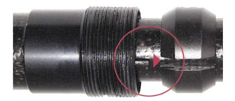
If you unscrew the hand nut by more than 5 turns, the pin can come out of its location in the ring. Then when the screw lock is retightened, the pin may move away from its slot and will be bent or broken by the compression ring.
