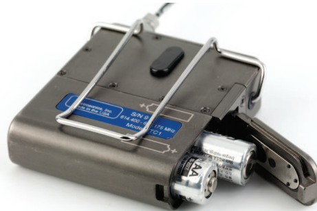
A machined aluminum, hinged door maintains reliable battery contact.
